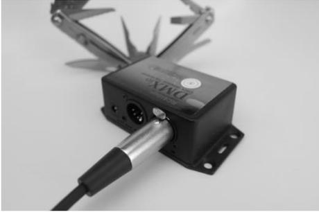
RC4Magic-900 devices work reliably to 800 feet (243m) or more outdoors, and marginally less indoors. The DMXio is easily configured as a transmitter or receiver with the push of a button, and remembers this and other settings on every power-up.
