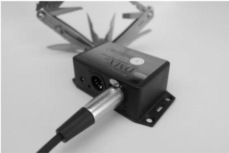
RC4Magic devices work reliably to 200 feet (65m) or more inside theatres and other performance spaces. The DMXio is easily configured as a transmitter or receiver with the push of a button, and remembers this and other settings on every power-up.
